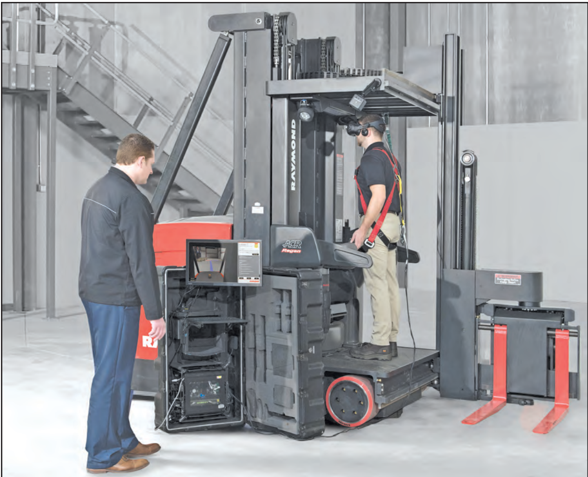
The Raymond Virtual Reality (VR) Simulator serves as a supplemental tool to assist in the education of new and existing forklift operators. (Submitted photo)
