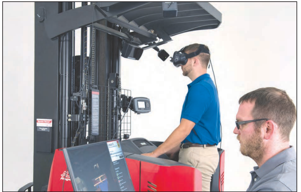
The Raymond Virtual Reality Simulator allows operators to become familiar and comfortable with the forklift and its controls prior to operating within the physical warehousing environment.
