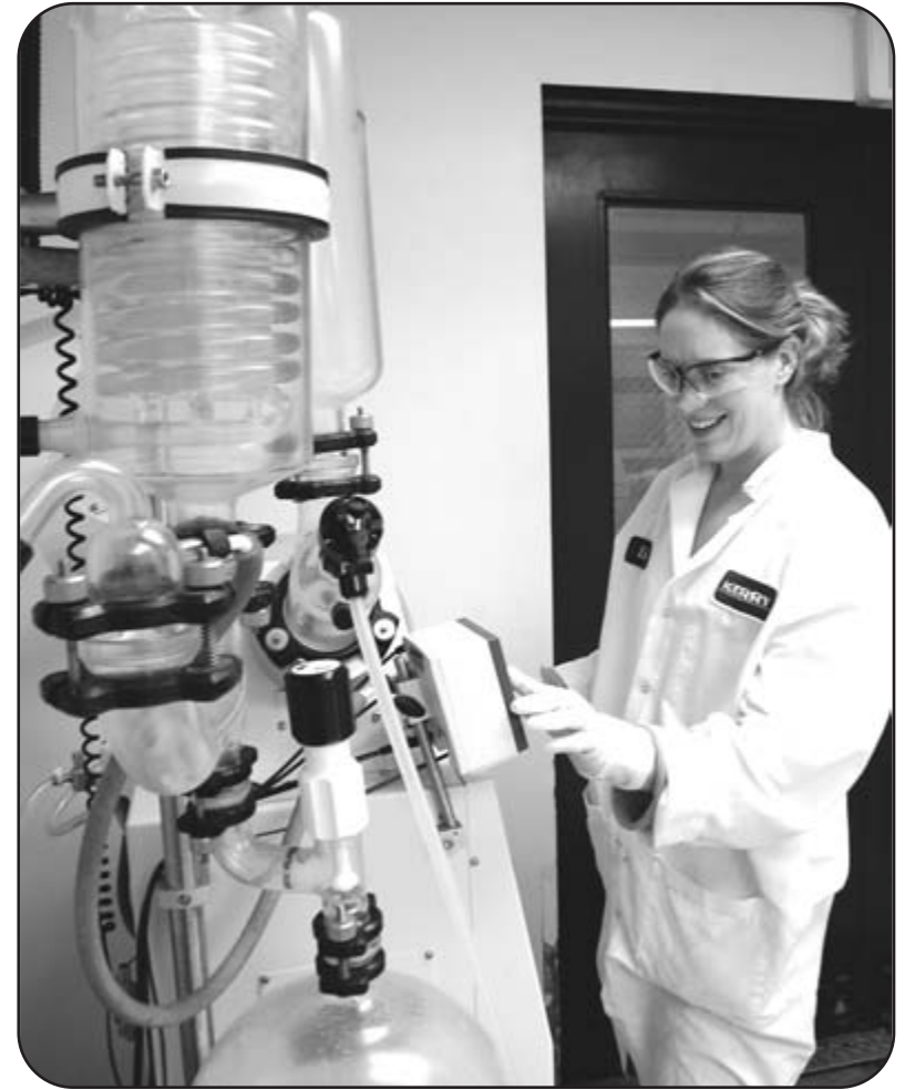
Product Development Scientist Lisa Hagen checks a pilot evaporator at a lab inside Sheffield Bio-Science in Norwich.
